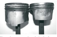
The piston on the right is from our "low friction" 9-5 and the one on the left is from a 1985 900T. Note the position of the piston rings and compare the size of the piston skirts. Less contact with the cylinder wall makes for low friction but it allows less heat transfer to the engine block which has to raise the temperature of the piston.
