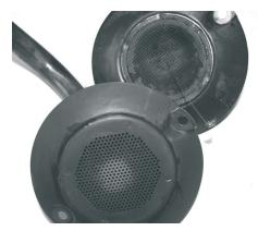
Oil pick ups. The top is from a 9-5 with a .026 wire in the mesh. The bottom is from a 9000 with holes that are larger. One of our first solutions for the 9-5 lubrication problems was maybe a bigger mesh in the screen but we soon discarded that idea when we saw the pump construction. All photographs by the author.
